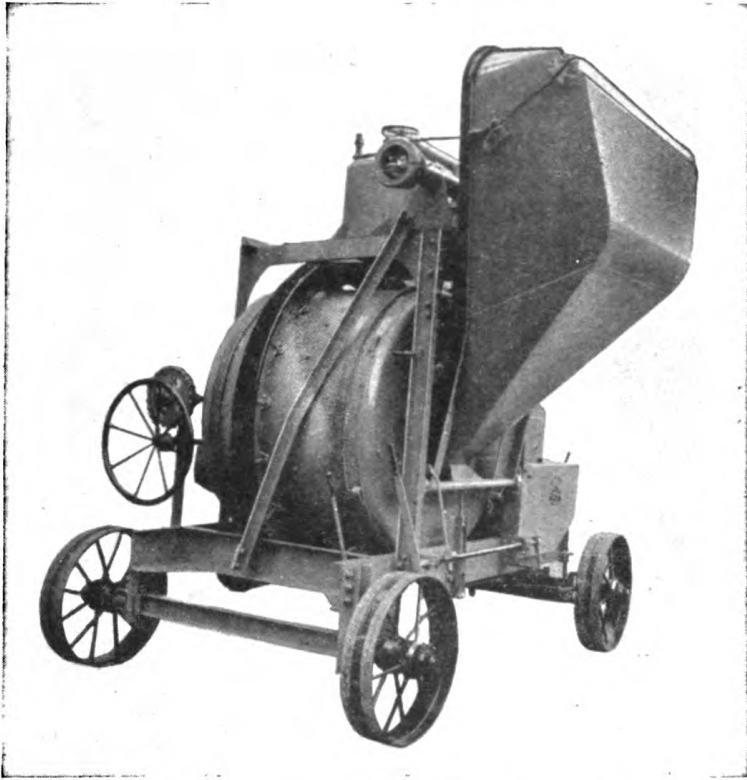
Figure 214. Mixer, concrete, gasoline-engine-driven, trailer-mounted, 14-cubic foot.
